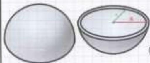
$$Q = \frac{4\pi K (r_1 + r_2) (T_1 - T_2)}{r_2 - r_1}$$
